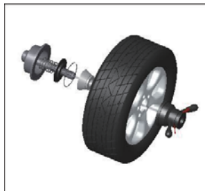
Main shaft-suitable cone(big head towards inside) —wheel—quick handle nut
